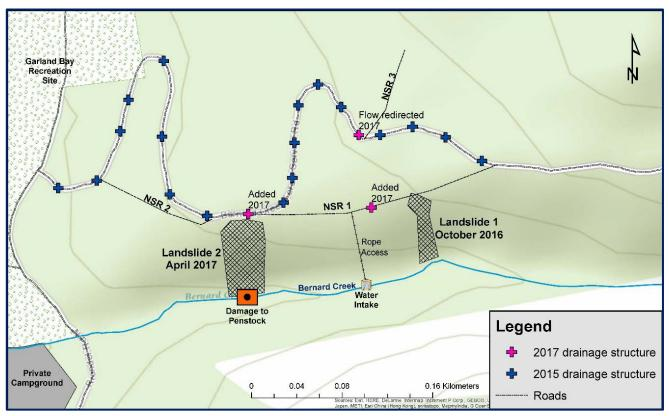
Figure 2. Location of landslides, water intake and drainage structures.
