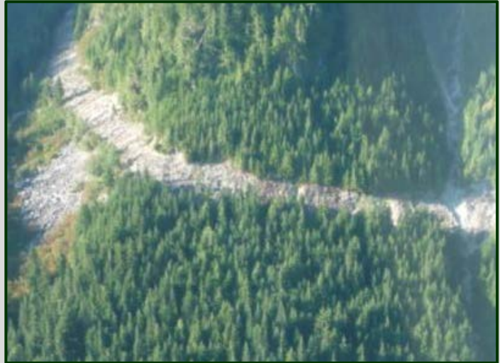
Figure 6. This photo shows a segment of road in watershed #9 that has been permanently deactivated by MFLNRO.
