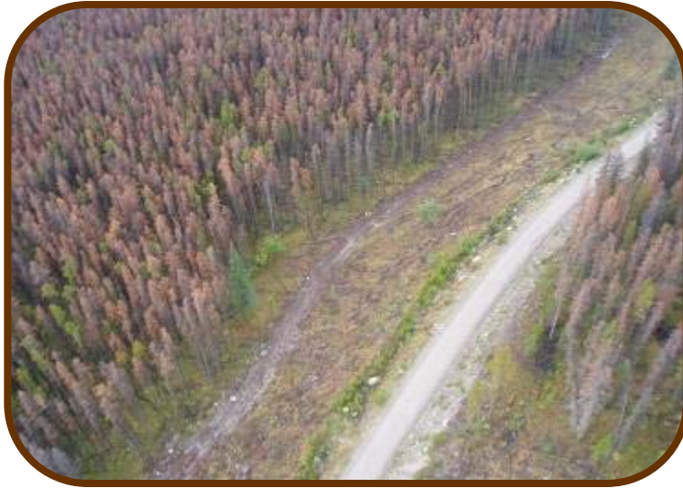
Figure 5 – Right-of-way danger tree removal.
