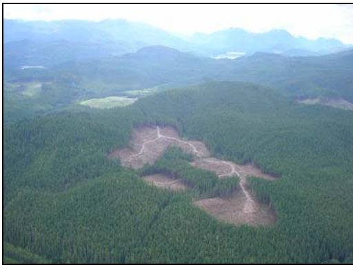
Harvest design is used in conjunction with on-ground treatments to minimize impacts of windthrow. The large retention area in the middle of this block was kept in order to reduce "fetch distance" to the edge of the harvest block, which is adjacent to a provincial park.
