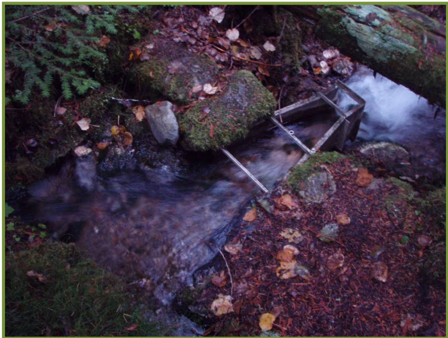
Device used for measuring water flow, Carter Creek.
