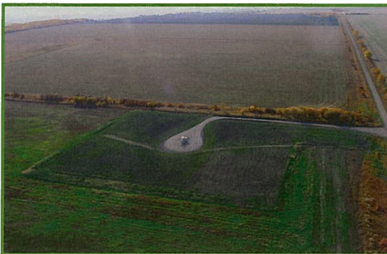
This well site has been "tear dropped", enabling farming to continue. Note access is along the field edge to minimize disruption to cultivation
