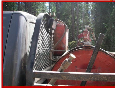
FIGURE 3. Hand-tank pump mounted on a headache rack.
