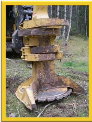
FIGURE 7. A feller-buncher head. The rotating saw blade can create sparks when it strikes a rock.
