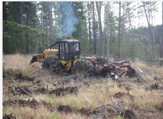
FIGURE 2. Disc trenching is a high risk activity.
