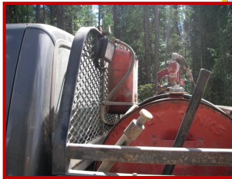
FIGURE 3. Hand-tank pump mounted on a headache rack.
