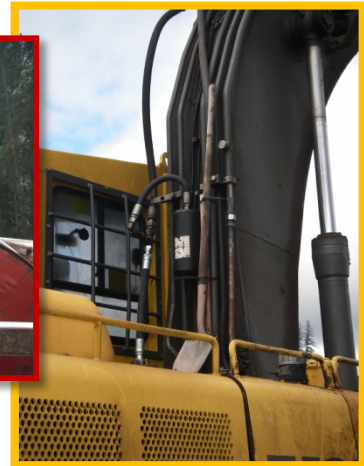
FIGURE 4. Shovel mounted directly to a feller buncher.
