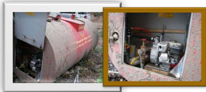
FIGURE 11 & 12. Portable water tank with a compartment for pump, hose and fittings ( left ). Close up of the pump in picture ( right ).
