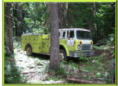
FIGURE 9. Retired municipal fire truck used as part of a fire-suppression system.
