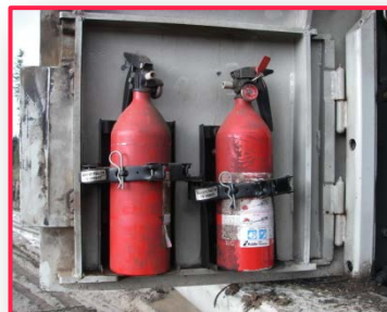
FIGURE 13. Fire extinguishers mounted on an excavator.
