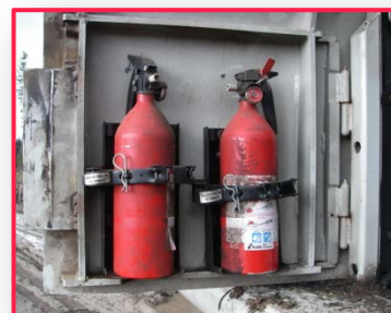
FIGURE 13. Fire extinguishers mounted on an excavator.
