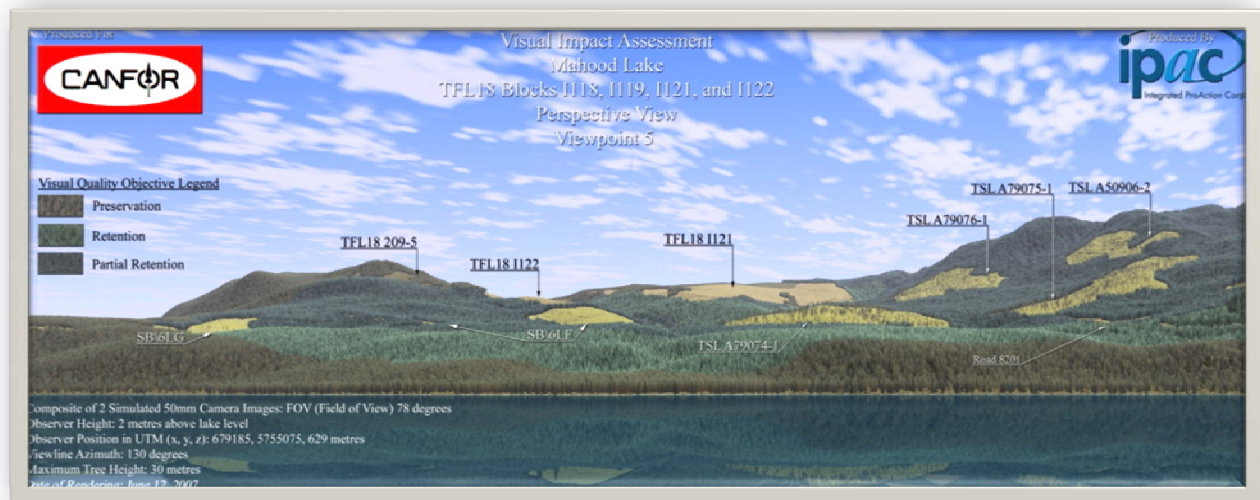
FIGURE 4. An example of a modelling technique where operators simulate proposed forest cover alterations to measure percent alteration and assess design techniques in visually sensitive areas.
